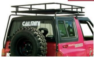
Only from CALMINI, a REAL rack for the Sidekick/Tracker! Made from 1"x.095 tubing for maximum strength. Installation is a snap - requires drilling only 4 small holes. Works with soft top, or as shown with aftermarket hardtop. Allows you to carry up to 200lbs. of gear into the back country. Comes with complete hardware & instructions. Black powder coat finish. 89-98 Sidekick/Vitara 2 door only. Part #SK3802
