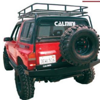
Mounts directly to frame and is bolt-on. 3/16" plate steel construction throughout and requires some minor welding to obtain maximum strength. One hand operation of swing away release. Reinforced ends for rock dragging. Carries a full size spare up to 33x12.50. Fits convertible and hardtop models 89-98 2 door only. For body-lifted models only. Shown with optional spin on tire release handle.
