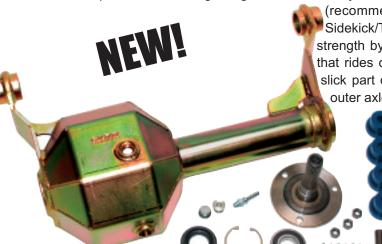
(recommended) third member housings from either Sidekick/Tracker or Vitara/Grand Vitara. We've built in additional strength by including a replacement passenger (short) side axle that rides on an outside bearing built into the housing. The real slick part of this conversion is that you use a drivers (left) side outer axle on both sides! You now only have to carry one spare!
